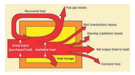
Figure 94. Heat lossed in a furnace
