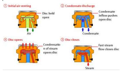
Figure 84. Operating principles of thermodynamic steam trap
