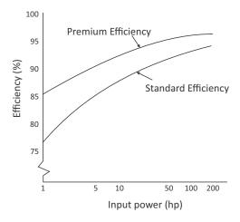
Figure 25. Standard efficiency motor vs. premium efficiency motor
