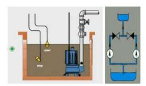
Figure 38. ON-OFF control for pump
