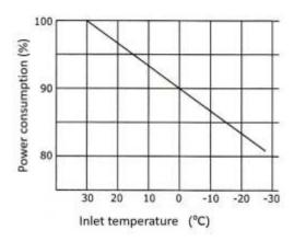
Figure 45. Effect of inlet temperature and power consumption
