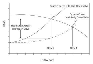
Figure 26. Performance curve of pump with flow control valve
