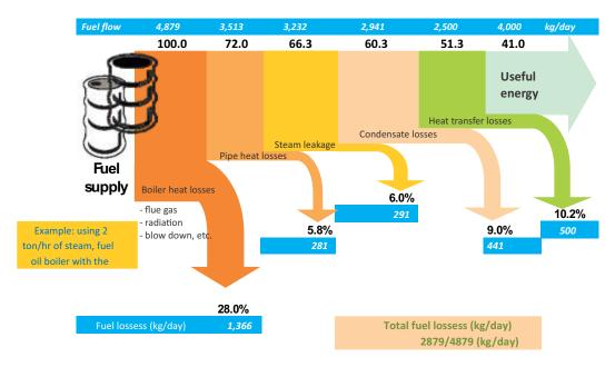
Figure 7. Sankey diagram for the energy loss in steam system
