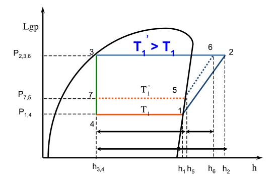
Figure 65. Relationship of the condensation temperature and the performance of the refrigeration
