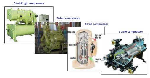
Figure 61. Basic types of compressors
