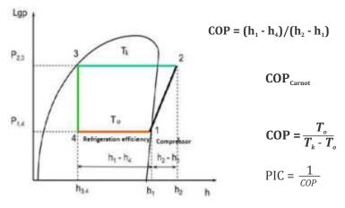
Figure 56. Calculation method of COP
