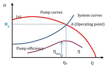
Figure 35. Pump Performance Curve
