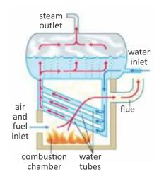
Figure 68. Simple diagram of Tube boiler
