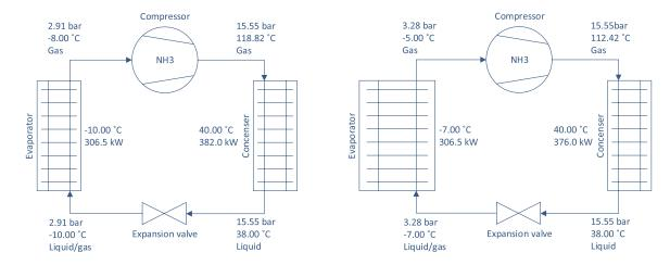
Figure 66. Principle schematic of two refrigeration systems with the different of the cevaporator temperature Source: LCTU (MOIT)
