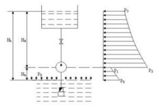
Figure 34. Parameters of Pump system
