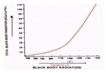
Figure 92. Black body radiation at different temperature
