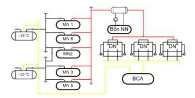
Figure 63. Diagram of Heat Recovery from discharge outlet from compressor
