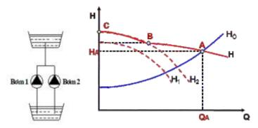
Figure 36. Parallel Pumps & pumps curve
