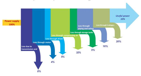
Figure 47. Sankey diagram for compressed air system
