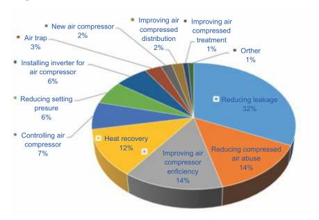
Figure 48. Energy savings potential for air compressed system
