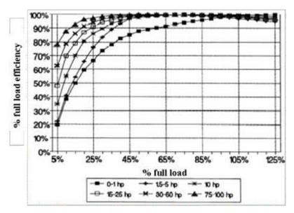
Figure 23. Efficiency and full load percent
