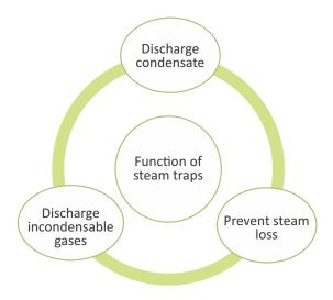
Figure 77. Functions of steam traps
