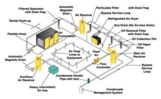
Figure 43. Air compression system illustration
