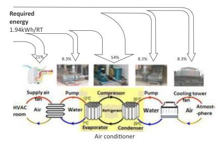
Figure 62 Typical heat transfer loop in refrigeration system
