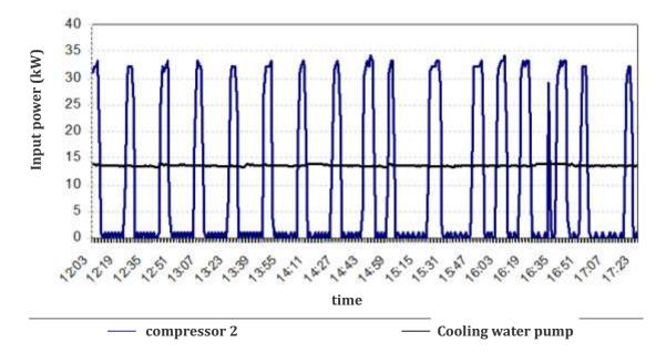
Figure 27. Load diagram of air conditioning
