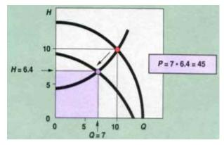
Figure 39. Performance curve of pump with VSD
