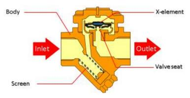
Figure 85. Thermostatic steam trap – Balanced pressure (source: TLV)
