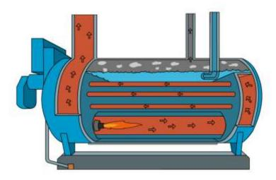
Figure 69. Fire tube boiler
