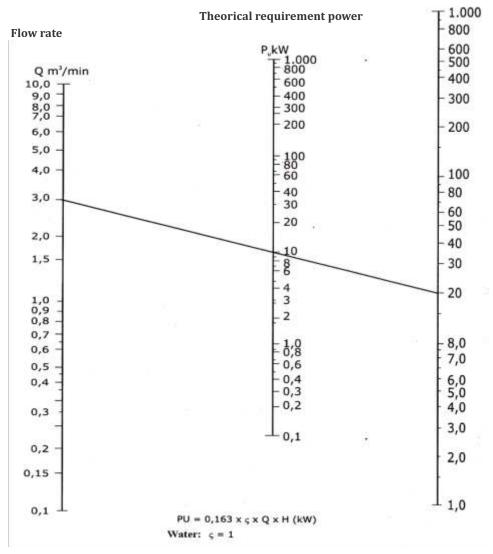
Figure 33 Calculate pump power
