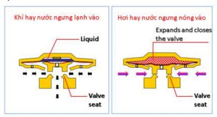
Figure 86. Operating principles of thermostatic steam trap – balanced pressure
