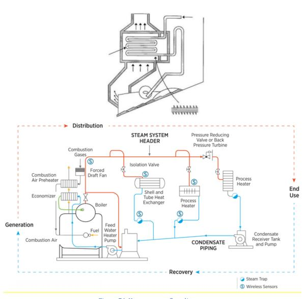
Figure 74. Heat recovery flow diagram
