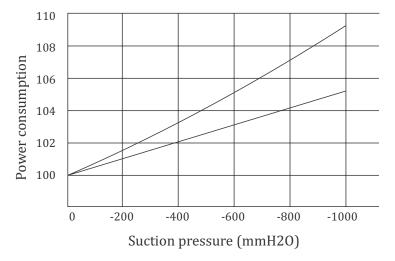
Figure 50. Effect of suction pressure and power consumption
