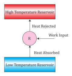
Figure 60. The refrigeration cycle
