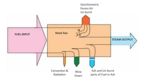
Figure 73. Sankey diagram of boiler
