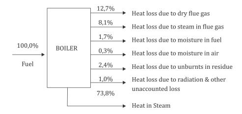
Figure 72. Typical losses from coal fired boiler
