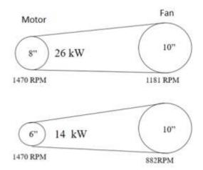
Figure 32. Reduce motor speed by decreasing the pulley size
