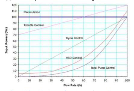
Figure 40. Power Requirements for various pumping control options
