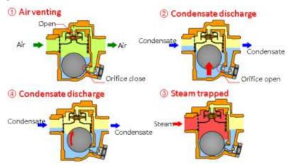
Figure 80. Operating principles of mechanical steam trap - Free float
