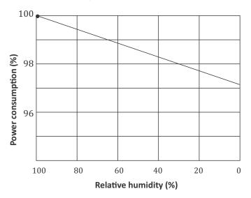
Figure 49. Effect of relative humidity and power consumption
