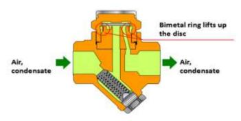
Figure 83. Thermodynamic steam trap (source: TLV)
