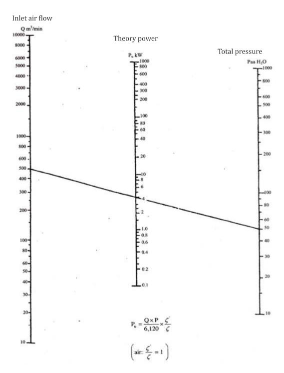
Figure 28. Fan power calculation
