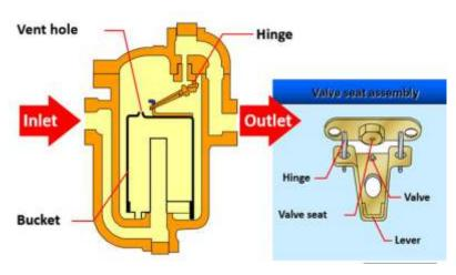
Figure 81. Mechanical steam trap – inverted bucket (source: TLV)
