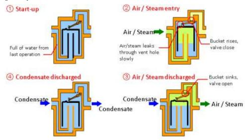
Figure 82. Operating Principles of mechanical steam trap – Inverted bucket
