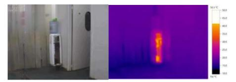
Figure 59. Detect heat sources inside HVAC space
