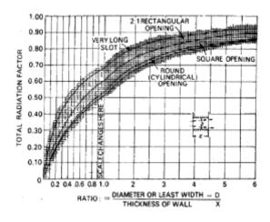
Figure 91. Radiation factor for heat
