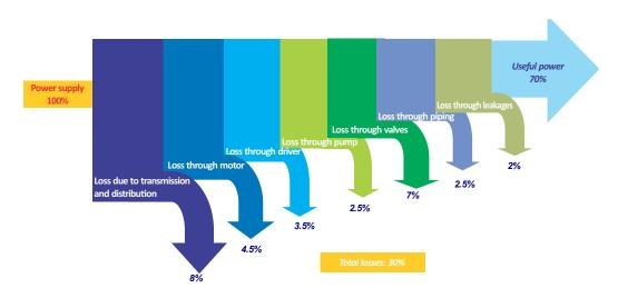
Figure 42. Sankey diagram of pump
