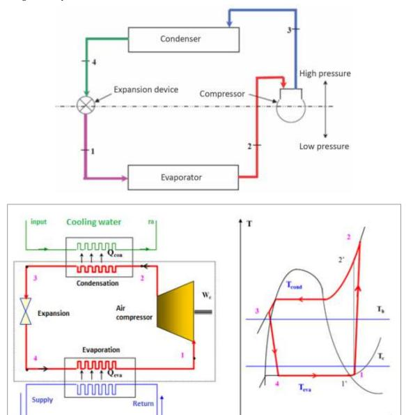
Figure 55. Operating Principles of air conditioner
