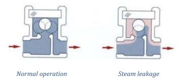
Figure 87. Steam trap operation
