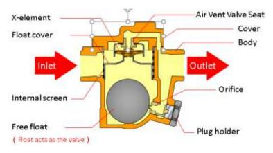
Figure 79. Mechanical steam trap – Free float (source: TLV)
