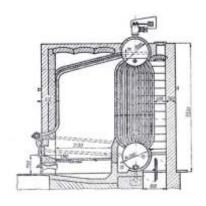
Figure 71. Water tube boiler with steam drum
