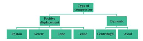
Figure 44. Type of air compressors
