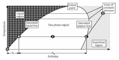
Figure 67. Steam phase diagram
