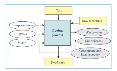
Figure 6. Flow chart of a dying process with energy and material flow
