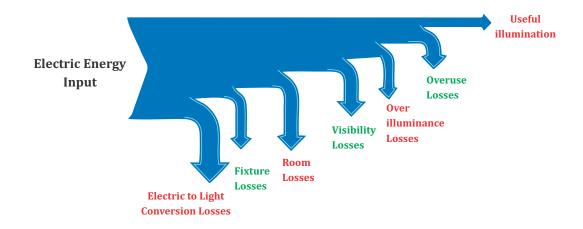
Figure 16. Sankey diagram of lighting system
