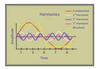
Figure 15. Waveforms of harmonics
